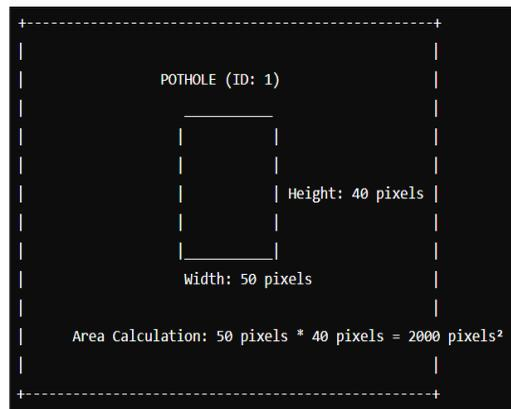
Figure 7. Wireframe image of pothole area calculation
