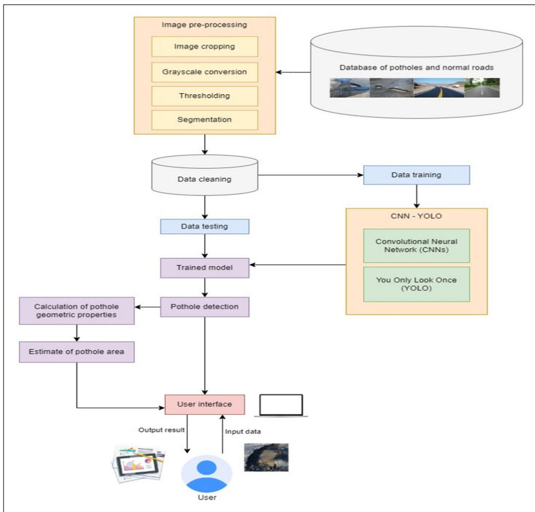
Figure 2. System architecture of pothole detection system
